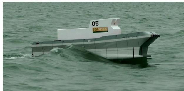
**Figure 6:** *Self propelled 1/12 scale model of SWATH craft tested at 25 knots at all headings in a 2.8m significant wave height sea-state. Motions recorded in all six degrees of freedom along with speed, propeller rpm, rudder angle and video data on and off the model.*
