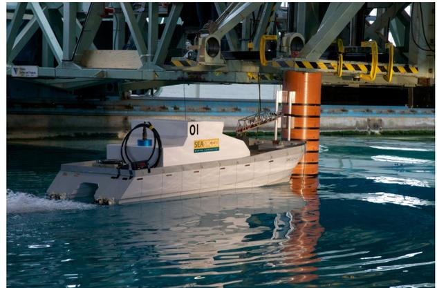
**Figure 8:** Self propelled scale model test of active motion compensated brow on a 24 metre WFSV hull whilst thrusting up against a turbine tower in head seas.
